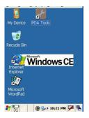
Of all the three indicating lights in the top right corner, the one in the leftmost will light after turning on, the middle one will turn to red after plugging in power, and turn to green after the battery is filled. For example, the red marker box in the above picture displays battery level and signal strength. Battery level indicate: Normal above 30%; insufficient 10%-30%; low power less than 10%.
